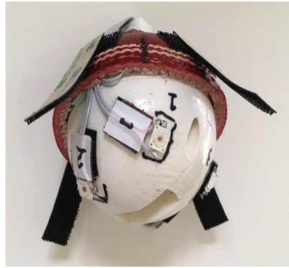
FIGURE 5. A 3D-printed core offers more flexibility for precisely embedding tiny LEDs inside the ball.
