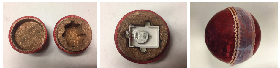
FIGURE 7. Impact-absorbing sensor case is fit into the ball and then sealed.
