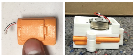
FIGURE 6. A shock-absorbing silicone rubber is used to wrap the sensor before embedding it inside a case.
