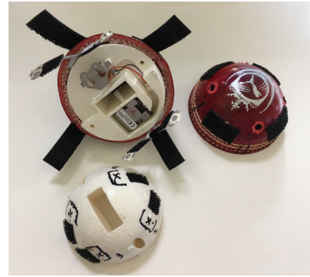
FIGURE 5. A 3D-printed core offers more flexibility for precisely embedding tiny LEDs inside the ball.
