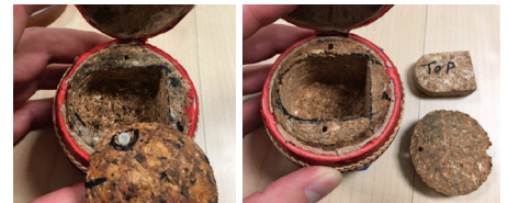
FIGURE 2. Space carved out of the wooden core for sensor embedding.
