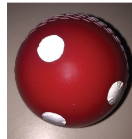
FIGURE 10. A cricket ball instrumented with IR tapes.
