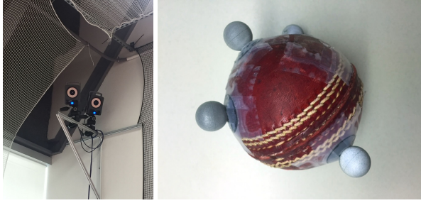
Figure 18: (a) IR based ViCon cameras at the ceiling. (b) A cricket ball instrumented with IR markers.
