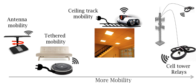
Figure 1: Regimes of infrastructure mobility, ranging from centimeter scale micro-motions, to feet scale mini-motion under couches, to building scale macro-motion on tracks laid on ceilings. In future, flying quadcopters could serve as cell-tower extenders to meet client needs.
